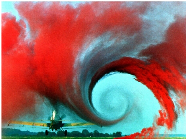
Visualization of wing tip vortex with colored smoke behind small airplane (NASA LaRC)
