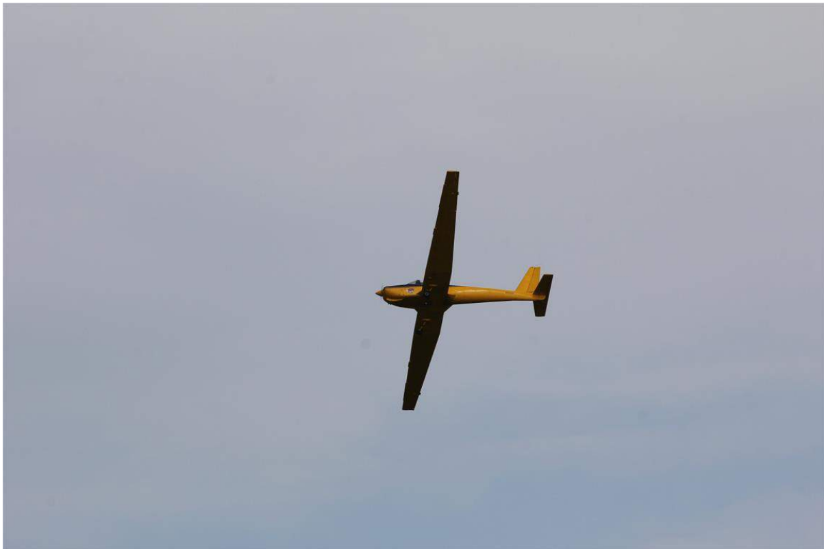
This is a Schweizer SGM 2-37 (TG-7A), a motor glider that is a combination of 1-36 and 2-32 parts, with the firewall forward installation from a Piper Tomahawk.
